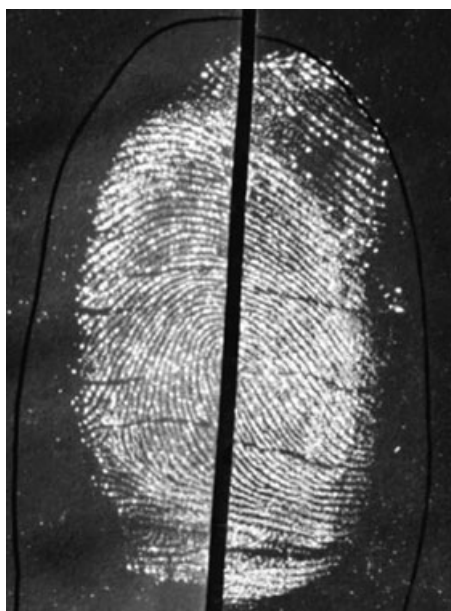
FIG. 3—White shopping bag (substrate 1) showing (left) 1,2-indandione (IND) and (right) IND-Zn developed latent fingerprint. Images recorded in the luminescence mode with, for both (left) and (right), excitation at 473–548 nm and observation using an OG549 long pass filter.
